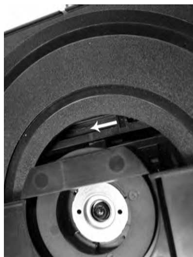
Manually opening of tray When it is not possible to open the tray with the EJECT button, the tray can manually be opened. When no disc is loaded, unlock the tray by moving the slide from left to right and pull tray outwards.
